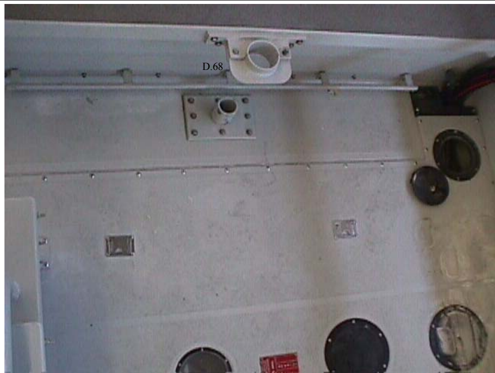
D.68. The TPSB has two M240B gun mounts. One mount is located on the starboard aft bulkhead and the second is located on the port aft bulkhead.
