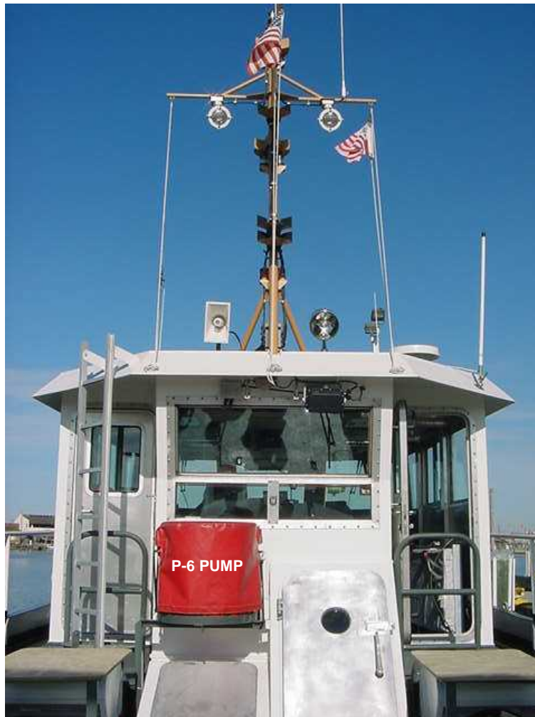
Figure 2-25 Emergency Dewatering Pump
