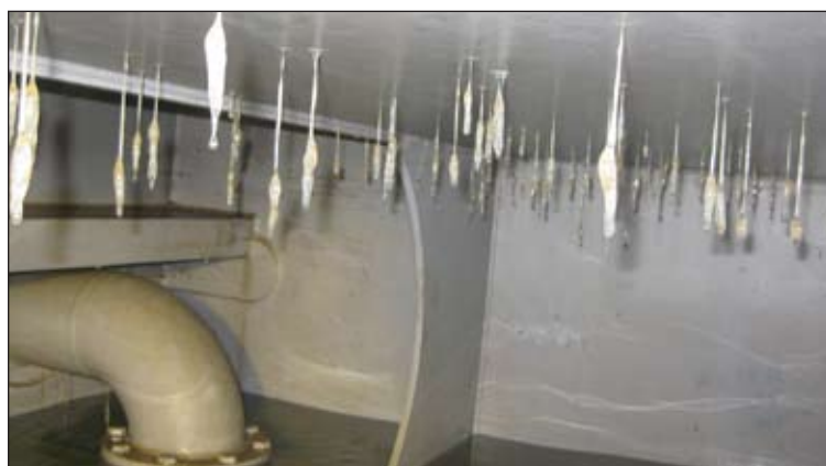
Tunicate organisms in a ballast tank of a cargo vessel in the Pacific Ocean (bottom).
