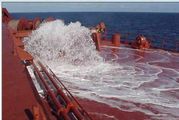
Water overflowing from a ballast tank deck hatch during ballast water exchange at sea (top).
