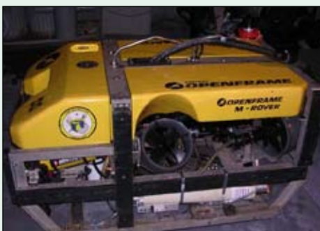
The University of Michigan's remotely-operated vehicle M-ROVER was used for mapping and sample collection in the 93-m deep Isolated Sinkhole.
