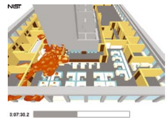
Computer animation showing flame iso-surface in office suite at 7 min 30 s after flaming ignition.
