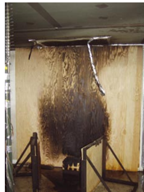
Two examples of results for fire test using sprinkler systems are shown. The top photograph demonstrates high wall wetting by the sprinkler, leading to rapid fire control with a single sprinkler in a corner test. The image below shows that flame extension occurred on the wall and ceiling for a wall test with two sprinklers in which the water flow was reduced below current design levels.
