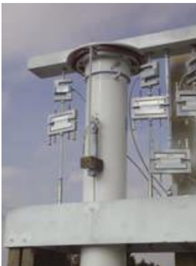
State-of-the-art field exposure apparatuses for naturally stressing sealant samples are positioned on BFRL's roof. Numerous physical and environmental variables continuously are being monitored, including stress and strain within the sealant while environmental variables, as well as sealant temperature and moisture content, are varied.
