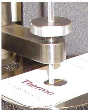
A useful technique for obtaining information on the molecular structure of polymeric materials is attenuated total reflectance (ATR) infrared spectroscopy, shown here in the process of analyzing a ballistic fiber bundle.
