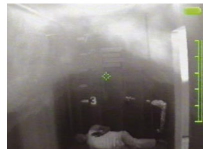
View of a corridor with a heated mannequin on the floor, and a temperature target and reflective strips on the back wall. Hot, smoke-laden gases are entering the corridor from an adjacent room on the right. The three TICs are viewing an identical scene at the same moment.
