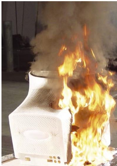
Photograph shows the burning of a monitor made from high impact polystyrene (no flame retardant).
