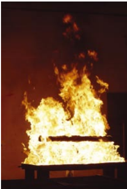
2.0 MW heptane fire from liquid spray burner.
