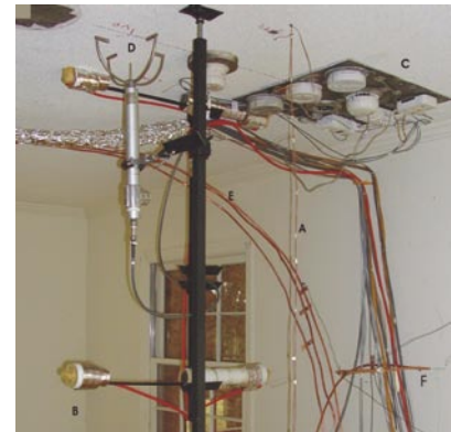
This photograph shows the wide range of instrumentation used to characterize the environment around smoke detectors during the recent investigation on home smoke alarms.
