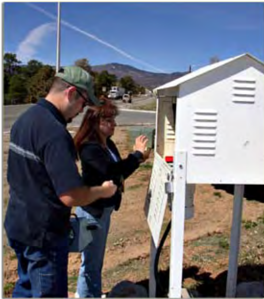
Technician taking measurements from an AIRNET station.
