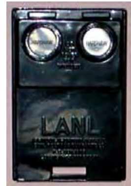
Thermoluminescent dosimeter (TLD) badge, like those carried by employees and used for monitoring outdoors
