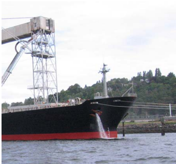
Water is pumped into vast tanks to stabilize a vessel, and later the ballast water is discharged. In this way, animals and plants can be transported thousands of kilometers from their native habitats and deposited in a new environment.
