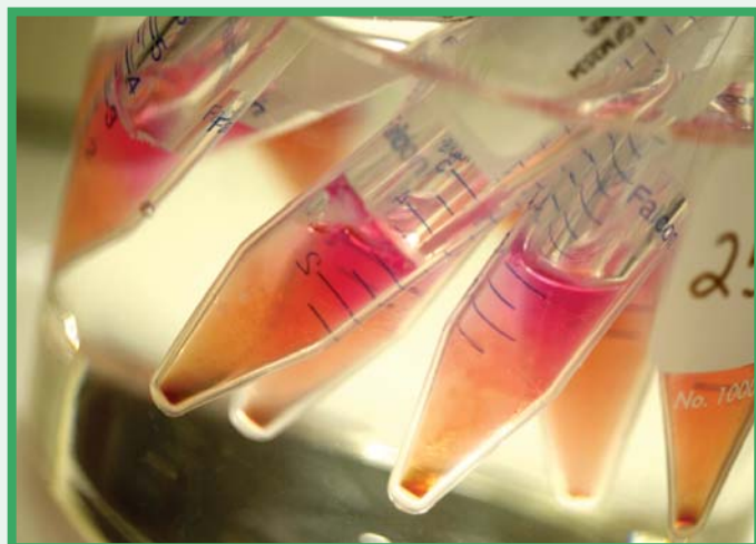
Vials of quantum dots and blood plasma following centrifugation, part of a study of the effects of quantum dots on immune cell function. Such studies are used to evaluate the safety of nanomaterials in humans. Computational methods could augment or replace these time-consuming and expensive laboratory tests. (Image courtesy of NCL).
