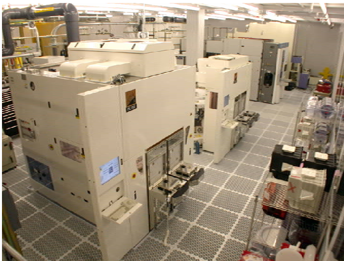
Figure 6.3. The 300 mm copper low-k dielectric process bay at the Advanced Tool Development Facility (ATDF), SEMATECH in Austin, Texas (courtesy of SEMATECH).
