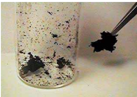
Figure 6.2. Single-walled nanotubes with \sim 1.4 nm diameter. Developing effective metrology that enables in-process measurements allows companies to take an important step toward achieving predictable product properties (courtesy of Paul McEuen, Cornell University).
