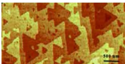
Figure 5.2. An example of an atomically ordered hydrogen-terminated silicon surface produced at NIST. These substrates can be subsequently used as catalysts for directed assembly and modified self-assembled structures (courtesy of NIST).
