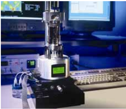
Figure 1.1. MultiMode Atomic Force Microscope for imaging small samples at high resolution (courtesy of Veeco Instruments).
