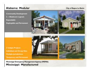
HUD code and local building codes. MS Eco Cottage is an energy-efficient unit that can also be used as permanent housing. Its design emphasizes green building technologies, durability, and an open interior design to accommodate families of various sizes.
