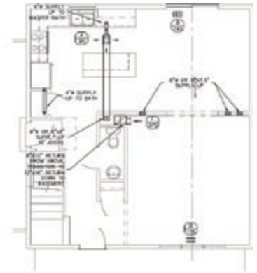
Show duct layouts on plans. (Source: CARB)
