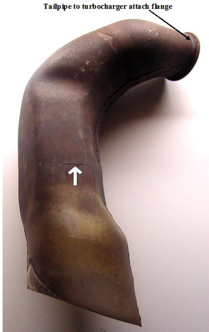
A tailpipe; with arrow pointing to crack through forward surface.
