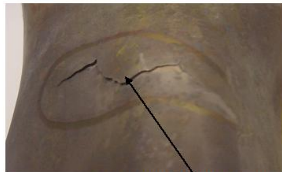
Crack through aft side of tailpipe
