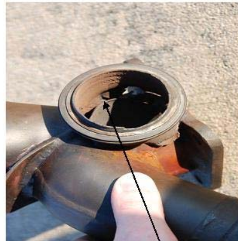
Photo 2: Wye waste-gate elbow attach flange fatigue failure.
