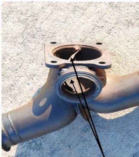
Photo 1: Wye, with failed internal baffle.
