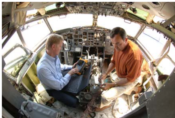
Mike Dinallo and Larry Schneider (left) prepare to employ the PASD diagnostic on a wiring bundle in the cockpit of a retired Boeing 737 at Sandia's FAA Airworthiness Assurance NDI Validation Center.
