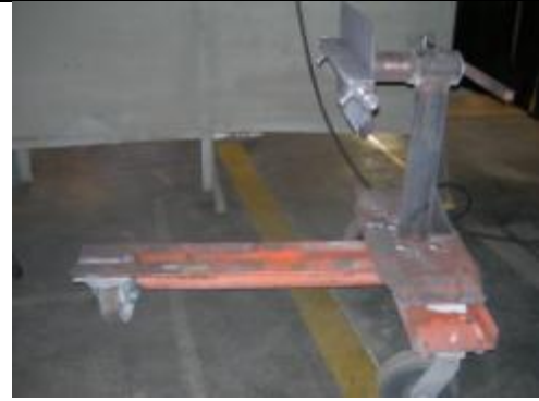
Figure 38: Accommodation ladders shop-workers designed a fixture to support and rotate accommodation ladders during welding and repair operations, MPHA program working with the accommodation ladder and watertight fitting shop to improve concept design and functionally through engineering.
