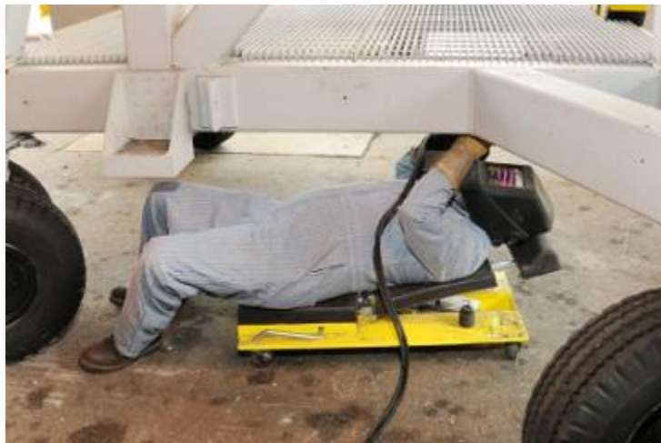
Figure 43: After: Welder is in a supported poster and can easily see the work piece
