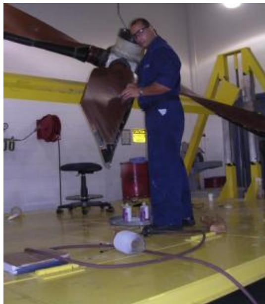
Figure 40: Fixture is height and angle adjustable
