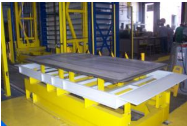
Figure 18: Vertical sheet metal storage system
