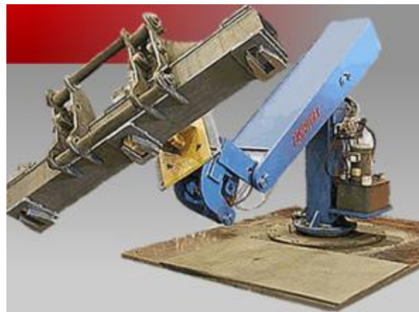
Figure 33 Rotating manipulator allows pieces to be held and manipulation in every direction. Mobile
