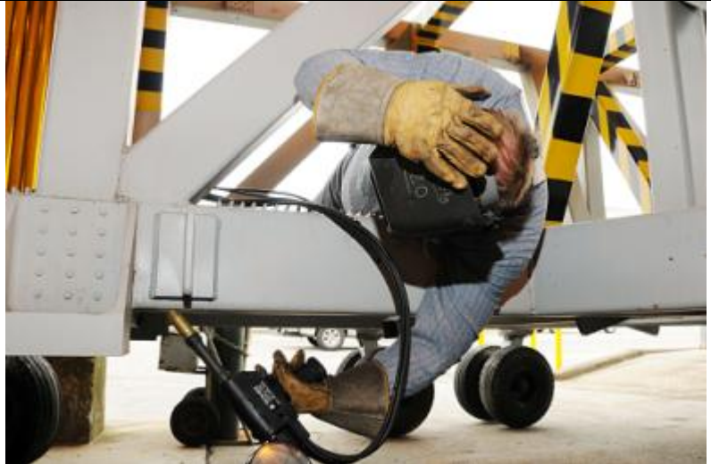
Figure 42: Before: Welder is in awkward posture to reach beneath work piece
