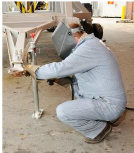
Figure 37 After: Simple trailer jack lifts work piece and improves posture at Fleet Readiness Center East
