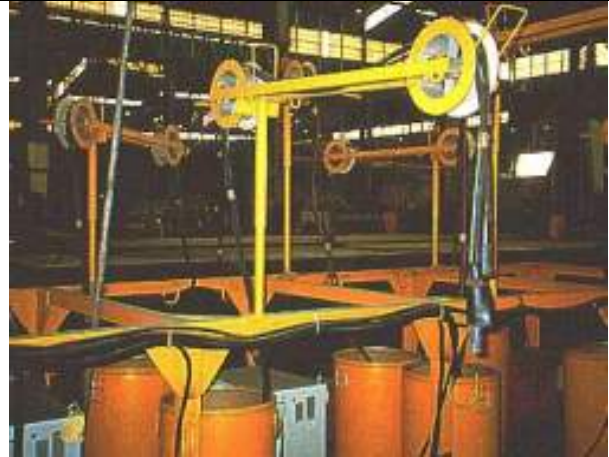
Figure 21: Welding lead on a pulley help to reduce awkward postures
