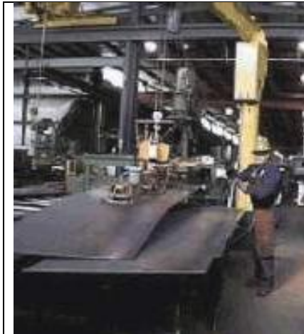
Figure 22: Suction manipulator used to move sheet metal
