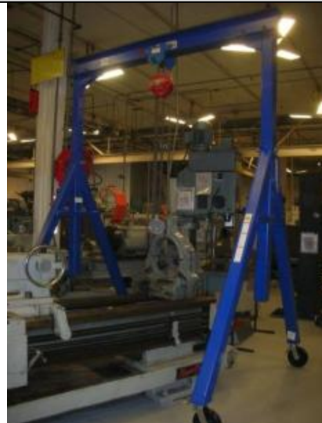
Figure 23: Southeast Regional Maintenance Center- portable gantry is used for raw material, moving dies, and finished products
