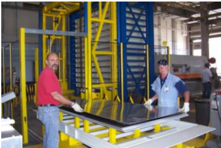
Figure 17: Vertical sheet metal storage system used at New London, CT
