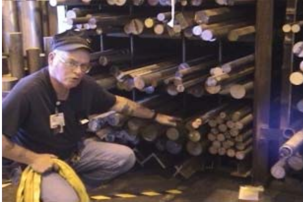
Figure 19: Before index unit, round stock retrieval was time consuming and required multiple pieces to be moved in order to locate the correct piece
