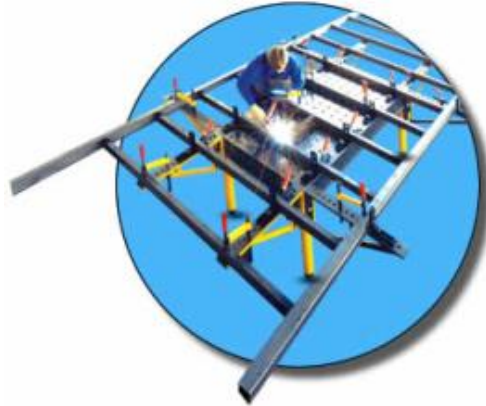
Figure 32 Welding tables can be joined together for larger parts and include clamping options to accommodate many sizes
