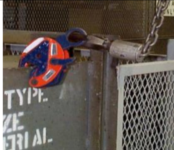
Figure 28: Grabbing clamp used at Naval Aviation Depot Jacksonville FL
