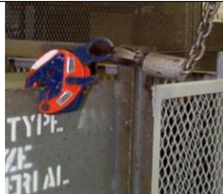
Figure 24: Grabbing clamp used at Naval Aviation Depot Jacksonville FL
