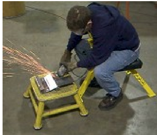
Figure 45: Welding stool supports torso and relieves some static muscle loading
