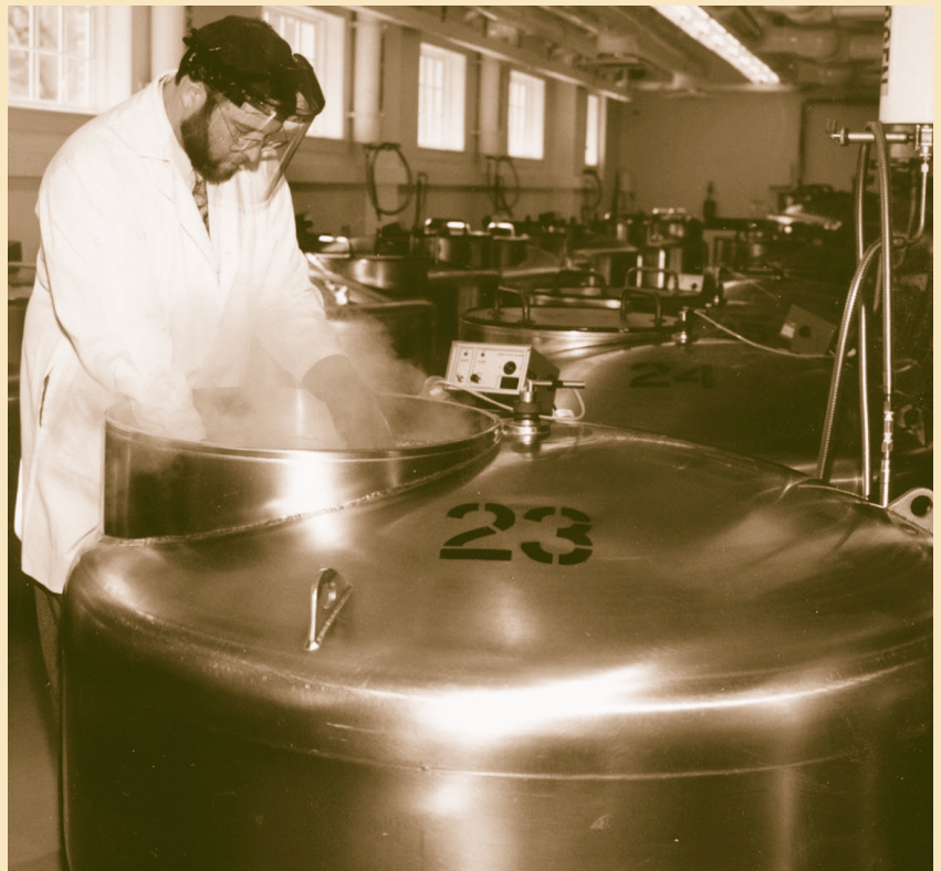
At the Coriell Repository tank room, cells are stored in liquid nitrogen and are preserved virtually indefinitely.
