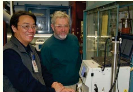
Mengdawn Cheng of ORNL and Emory Ford of Materials Technology Institute operate a differential mobility analyzer.
