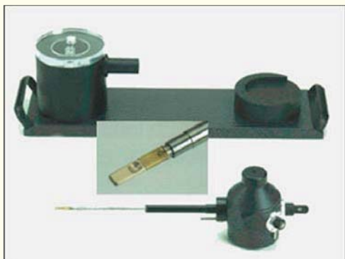
Fig. 2. Cryo-TEM cryostat used to load sample, holder tip where cryo sample is inserted; cryo-cooled sample holder.
