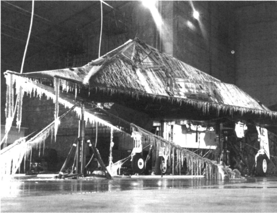
A F-117A Stealth aircraft undergoing icing tests in the main chamber of the McKinley Climatic Laboratory at Elgin Air Force Base, Fort Walton Beach, FL. The laboratory, whose period of significance extends to within the past fifty years, was listed based on exceptional importance for its contribution to the development of military aviation during the World War II and Cold War eras, and for its advanced engineering design. (Official U.S.A.F. photograph, 1991)
