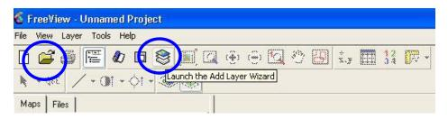
Another method – necessary when adding imagery – is to use the *Add Layer Wizard*. This option will require the user to make band assignments. In the first window of the Wizard, the user selects the type of layer to add.
