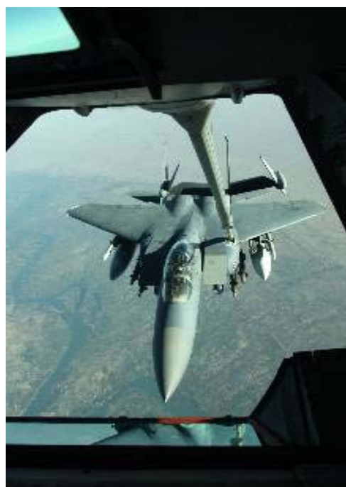
An F-15E Strike Eagle receives fuel from a 908th Expeditionary Aerial Refueling Squadron KC-10 Extender during a mission over Iraq. U.S. Air Force photo by Senior Master Sgt. Mark Moss
