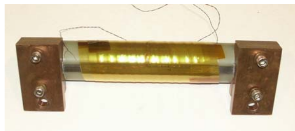
Fig. 2.40. Sample holder for burnout current testing of HTS conductors in a liquid nitrogen bath
