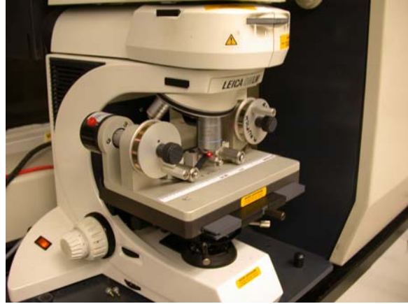
Fig. 1.17. Reel-to-reel device used to feed and control long-length coated conductor tape specimens during Raman microscopy examinations. The device is shown in position on the microscope stage of the Raman microprobe.
