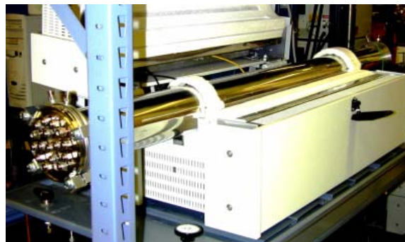
Fig. 1.76. The reduced-pressure chamber that sits in the cradle of a tube furnace.
