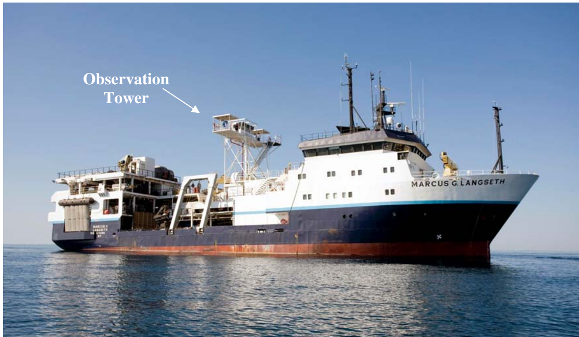
FIGURE C.1. The source vessel, the R/V Marcus G. Langseth , showing the location of the observation tower from which visual observations for marine mammals were made.
