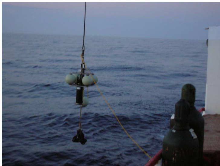
Figure 1. An OBH system being deployed.
