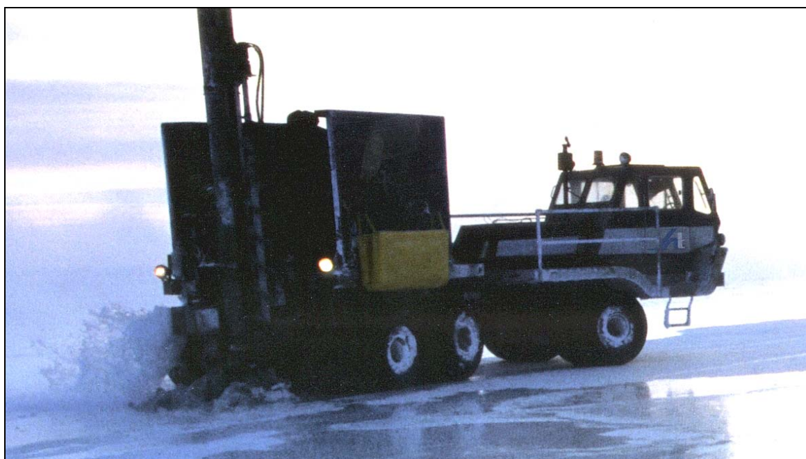
FIGURE 1.6. Blue Bird rolligon-type vehicle with 12" ice auger (stowed) and 10.2" pump auger (in use).
