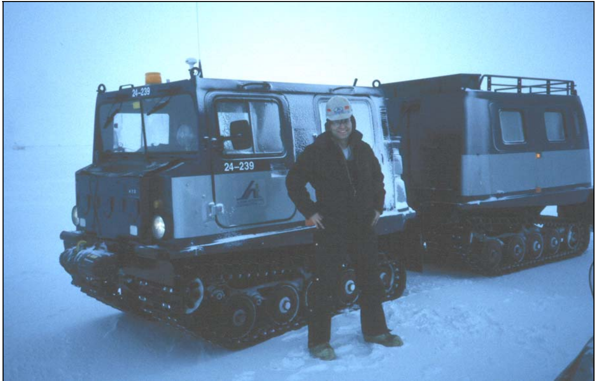
FIGURE 1.3. Hägglunds tracked vehicle and personnel carrier. Power is from a turbocharged diesel engine capable of 143 hp at 4600 rpm; total weight of the two cars is ~4536 kg (10,000 lb).
