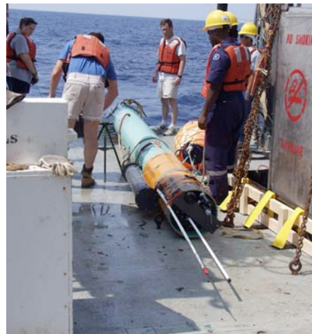
FIGURE 3.1. The spar buoy used to measure sound levels of the various airgun arrays (photograph by J. Diebold).
