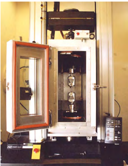
PBX materials have been tested to failure quasi-statically in uniaxial compression and tension under various conditions. Shown here is the Instron workstation and chamber, along with pre- and post-test compression (right) and tension (left) PBX 9502 specimens.
