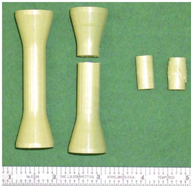
PBX materials have been tested to failure quasi-statically in uniaxial compression and tension under various conditions. Shown here is the Instron workstation and chamber, along with pre- and post-test compression (right) and tension (left) PBX 9502 specimens.
