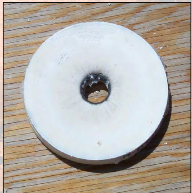
PBX-9501 damaged from the impact of a projectile fired at 430 m/s (low velocity).
