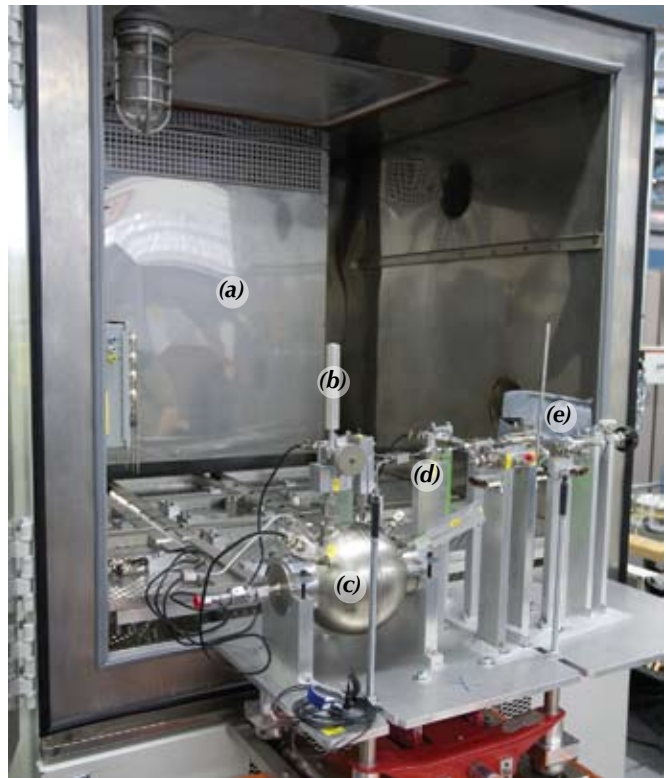
(a) The environmental chamber for our VSTS II. The apparatus in the foreground is our VSTS II showing (b) the gas sample bottle, (c) the test pressure manifold receiver vessel, (d) the valve under test, and (e) the source vessel. The system includes pressure transducers and temperature probes for gas volumes and vessel surfaces.
