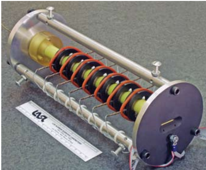
This figure shows a photo of an actual experiment and the associated detonation shape record. The photo ( left ) shows an 18-mm-diameter front-curvature rate stick that is designed to accommodate a wide range of initial temperatures. The photo ( right ) shows the corresponding streak camera negative image. The mirror destruction technique gives a very crisp image, a necessity for effective DSD calibration.
