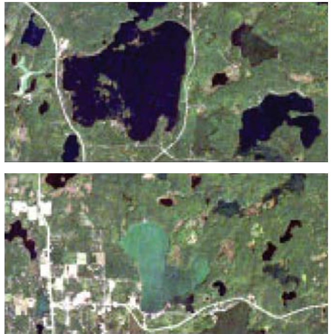
Figure A-7. Satellites can image a much wider area than can be effectively monitored from the ground. This pair of true-color Landsat images compares a clear, clean lake (top) with a lake with poor water quality (bottom). (Images courtesy Upper Great Lakes Regional Earth Science Applications Center) 12
