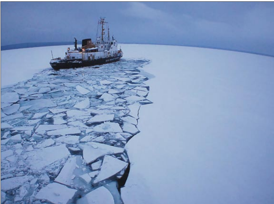
Coast Guard Cutter KATMAI BAY breaks ice for freighters navigating through the St. Mary's River in the Great Lakes. During winter, paths must be made in the ice for freighters to continue shipping goods.
