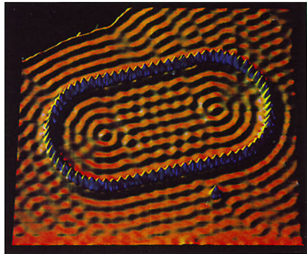
Figure VIII.3: An "atomic stadium" made visible by scanning tunneling electron microscopy. Iron atoms (shown in blue) form the walls of the stadium; the interior electron distribution is shown in orange.
