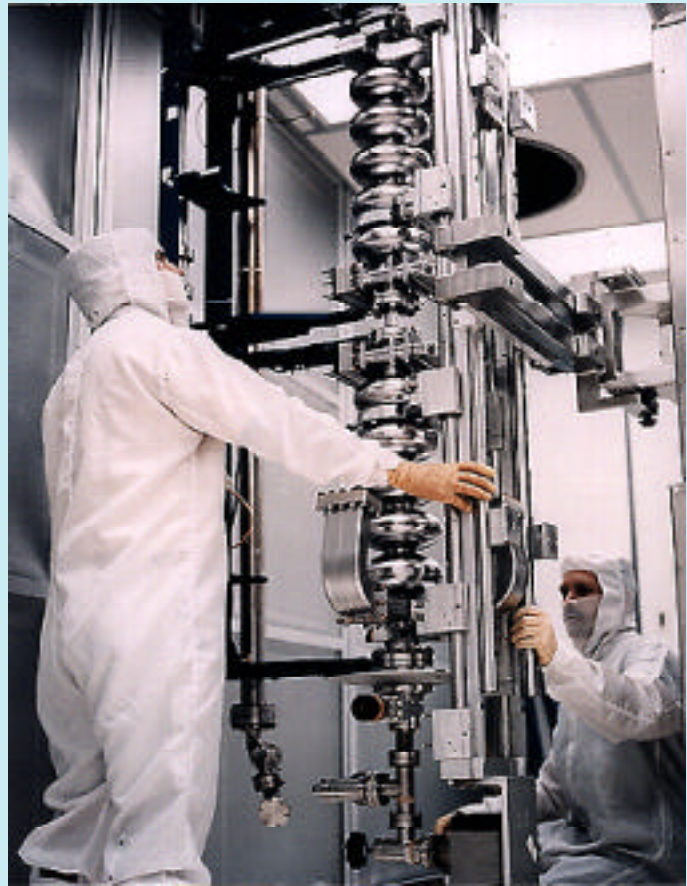
Figure II.C The world's largest assembly of superconducting accelerator cavities, cooled by a refrigerator that doubled the world's supply of helium at 2 degrees kelvin, are an essential element in the production of CEBAF's continuous electron beams.
