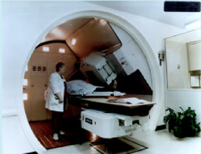
Figure VIII.A A medical technician aligns a patient in a superconducting cyclotron facility at Harper Hospital in Detroit. The compact cyclotron is being used for neutron irradiation of cancer and is based on the technology developed for research cyclotrons built at Michigan State University. Both the cyclotron and collimator for the neutron beam are positioned on the right about 45 degrees above the horizontal and can be moved to be at any angle relative to the patient.
