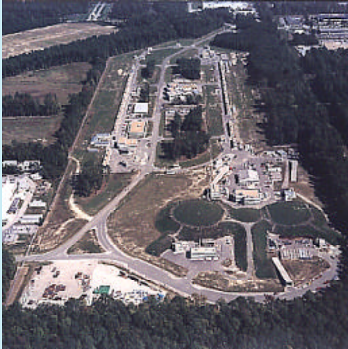
Figure II.D Aerial view of the recently completed Continuous Electron Beam Accelerator Facility (CEBAF). The electron beam traverses the mile-long, racetrack-shaped accelerator as many as five times, reaching an energy of 4 billion electron volts, and is then directed to the three large experimental halls buried under the circular domes visible in the foreground. The large building in the center of the racetrack houses the helium refrigerator.
