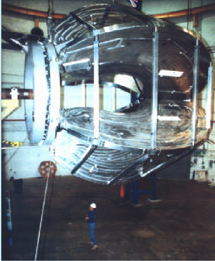
Figure V.B Large magnetic coils for CLAS, the novel detector which will permit new experimental studies of how quarks behave in nuclei when energy is delivered to protons and neutrons by the CEBAF electron beam.
