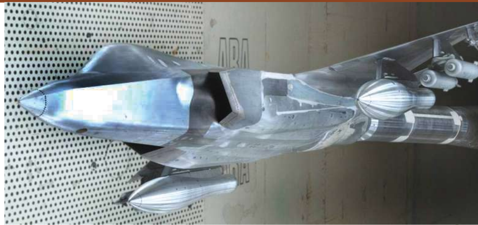
Lockheed Martin engineers coupled their high-fidelity computational fluid dynamics software with Sandia’s DAKOTA software to perform shape optimization of the F-35 fuel tank shape.
