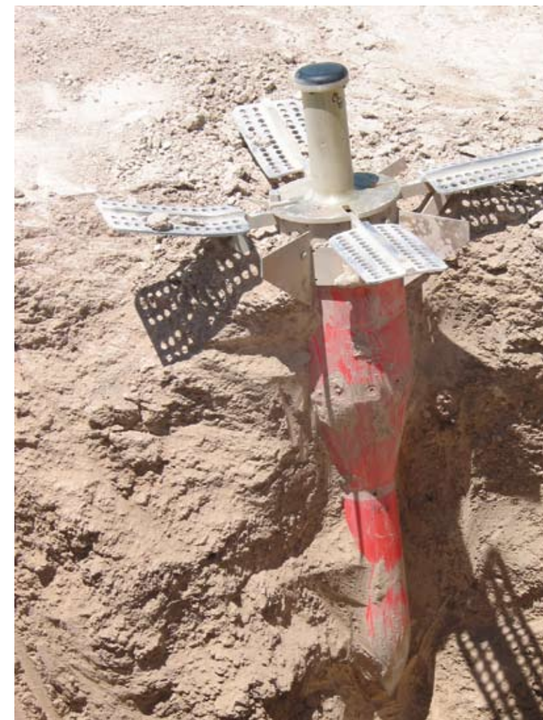
The second stage of the geological site-characterization probe transmits radio signals about geological data back to central communications.
