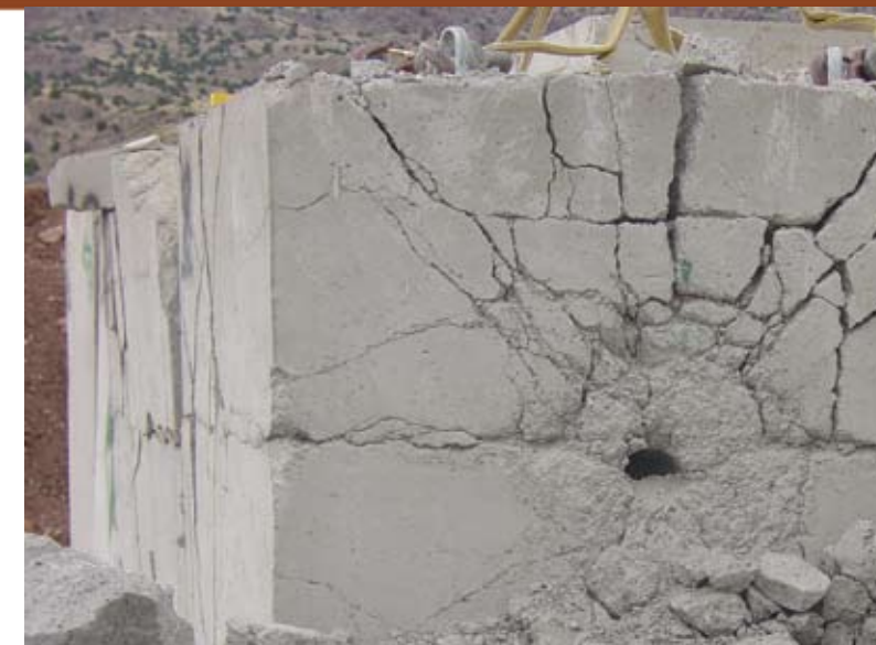
Post-test condition of a penetrator target, a series of concrete blocks, viewed after several penetrated target blocks were removed
