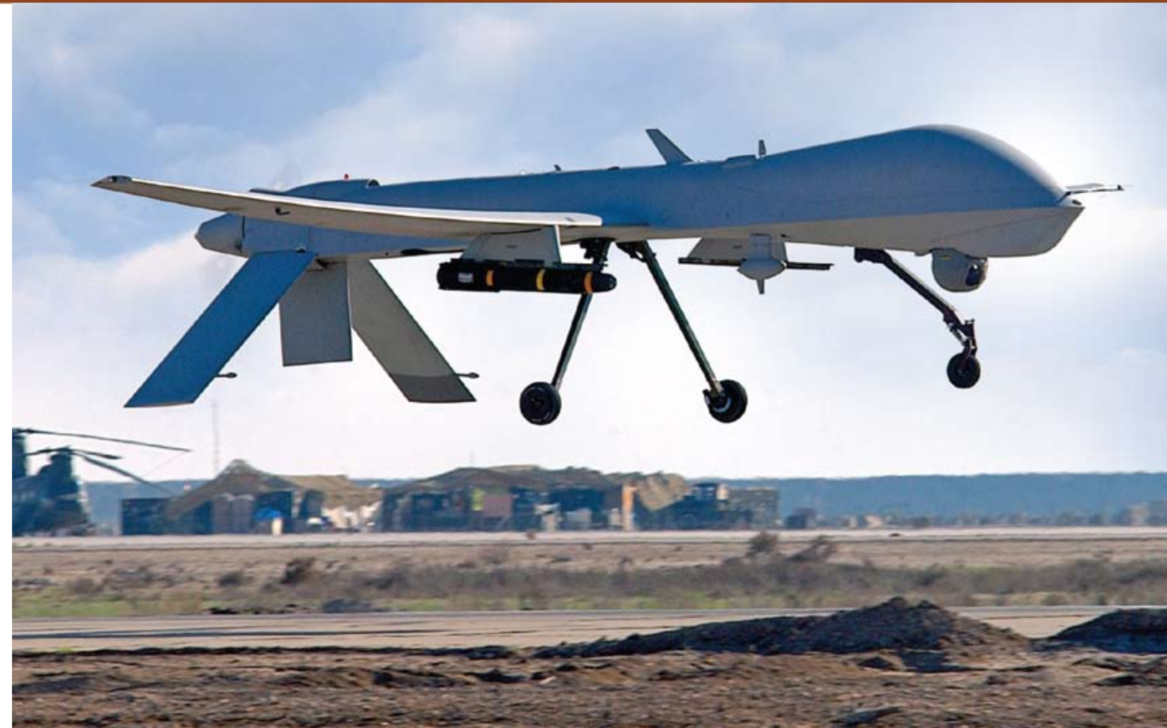
An MQ-1 predator, Unmanned Aerial Vehicle (UAV), exemplifying the type of carrier that might be utilized for current iterations of Sandia’s miniSAR radar package.
