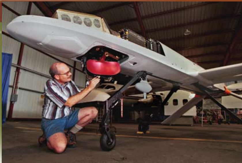
A Sandia staff member mounts a miniSAR package on an unmanned aerial vehicle.
