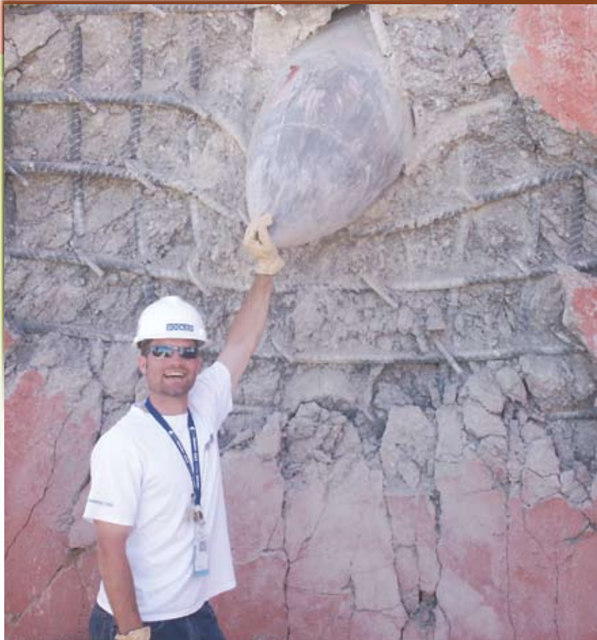
An illustration of the penetrator's potency through a wall of steel-reinforced concrete.
