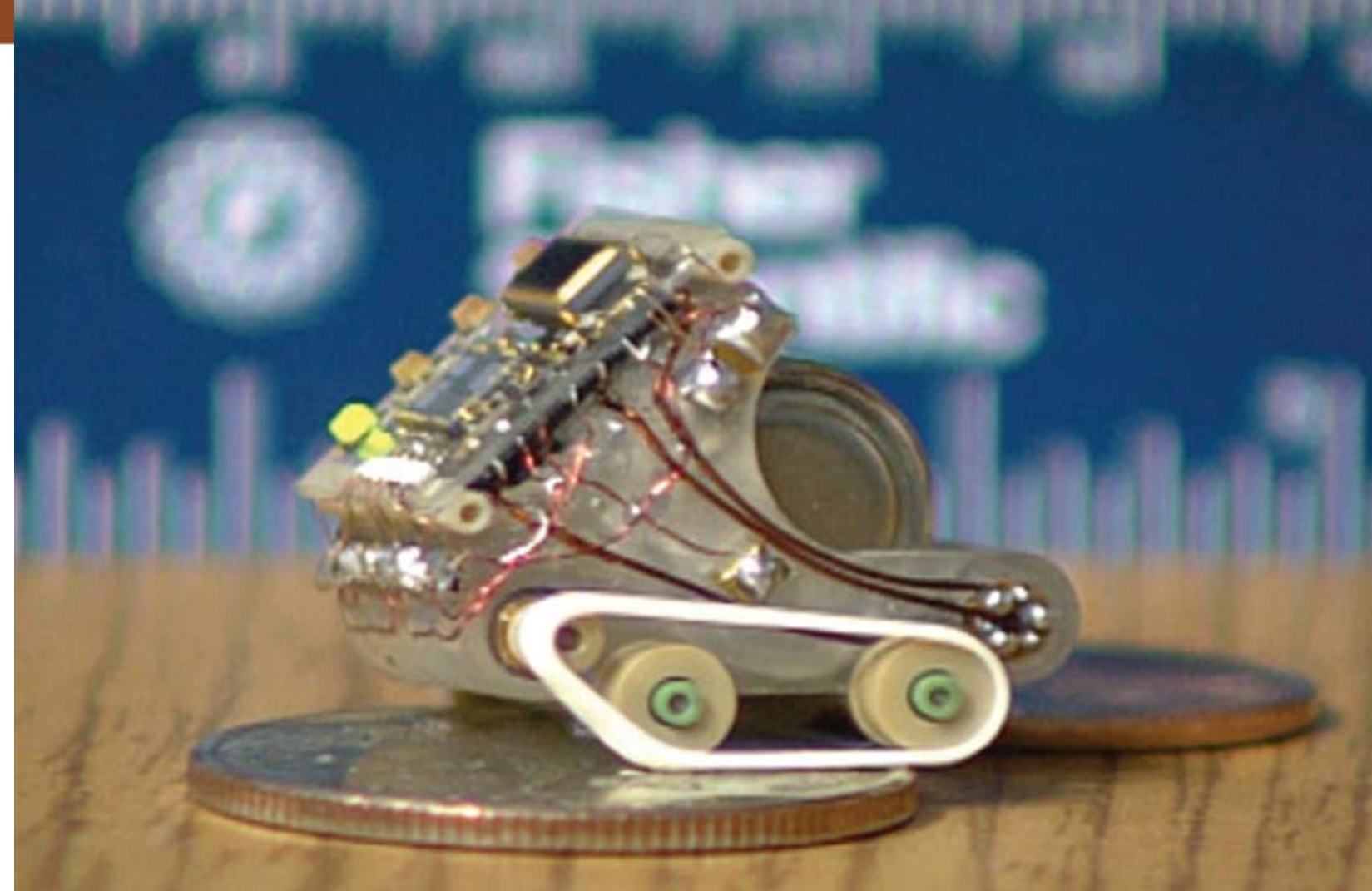
Sandia developed mini-robot, occupying 1/4 in 3 and weighing less than an ounce — possibly the smallest untethered robot ever created; MEMS inertial guidance offers the potential of fully autonomous operation.
