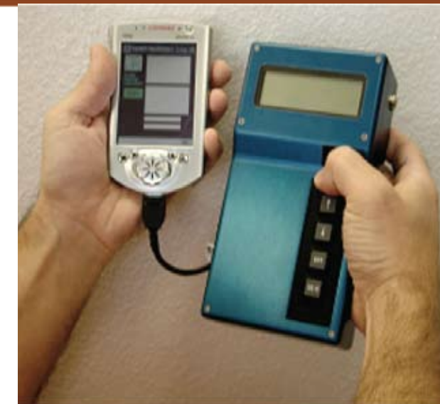
Microchemlab’s analytical data can be quickly downloaded to either a PC, or as shown here, even to a personal digital assistant (PDA).
