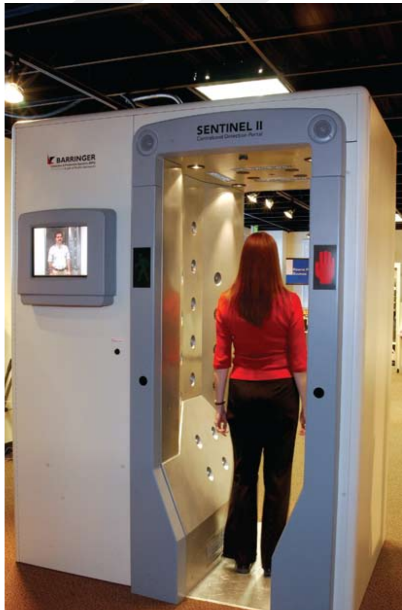
Sandia developed sample collection and preconcentration systems and integrated them with a commercial detector to build the first engineering prototype of this explosives detection personnel portal.
