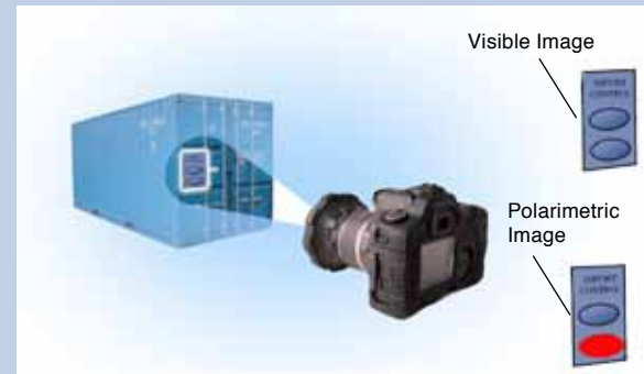
At-a-distance polarimetric imaging of radiation-sensitive tags on shipping containers.
