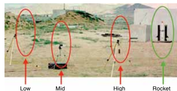
RF sensor system with low-, midrange-, and high-frequency antennas.
