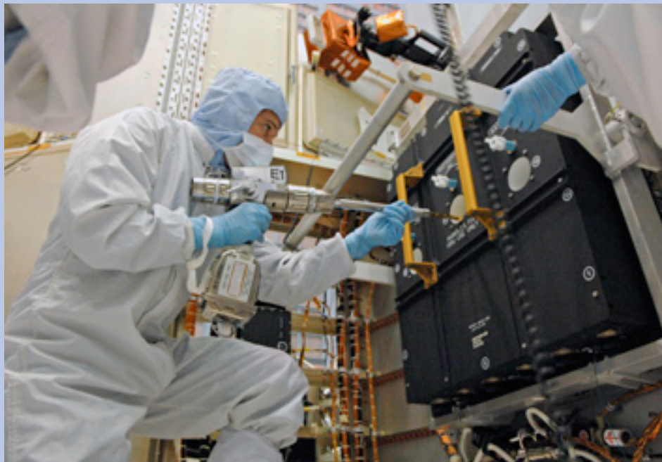
Caption: Mission specialist Michael Good practices installing a battery module into the Hubble High Fidelity Mechanical Simulator, located in the clean room at NASA's Goddard Space Flight Center.
