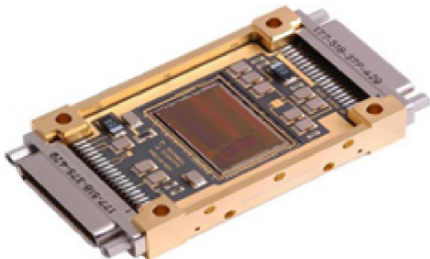
Caption: The SIDE CAR ASIC in spaceflight package.
