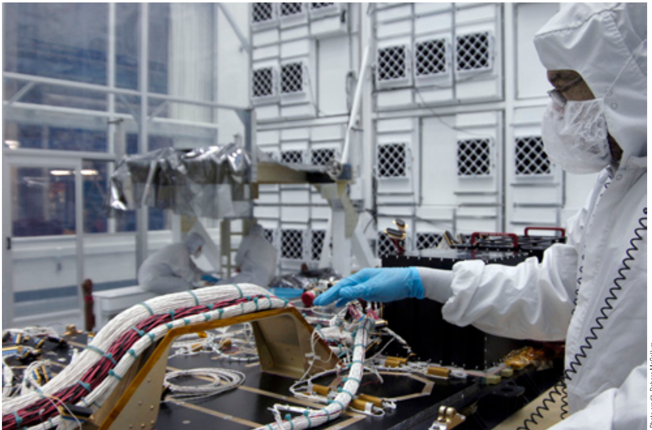
Caption: Command and Data Handling (C&DH) and flight Power System Electronics (PSE) are on the left. The gimbal control electronics are on the right, and the flight harness is all over the panel.
