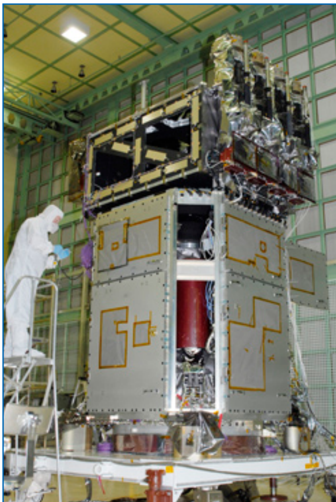
Caption: Solar Dynamics Observatory—Integrating the instrument module to the spacecraft bus.
