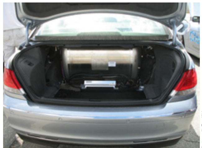
Caption: The vehicle's cryogenic tank stores 8 kilograms (kg) of liquid hydrogen at -250°C.
