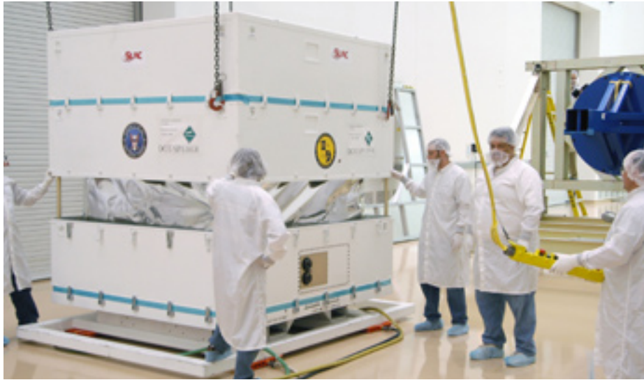
Caption: General Dynamics engineers prepare to remove the LAT from its shipping container after its arrival at the contractor's space systems facility in Gilbert, Arizona.
