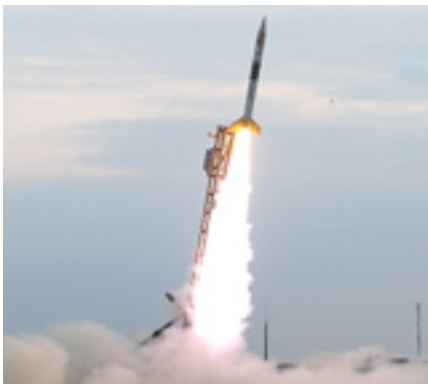
Caption: A NASA single-stage Orion sounding rocket carrying student experiments is launched from Wallops.
