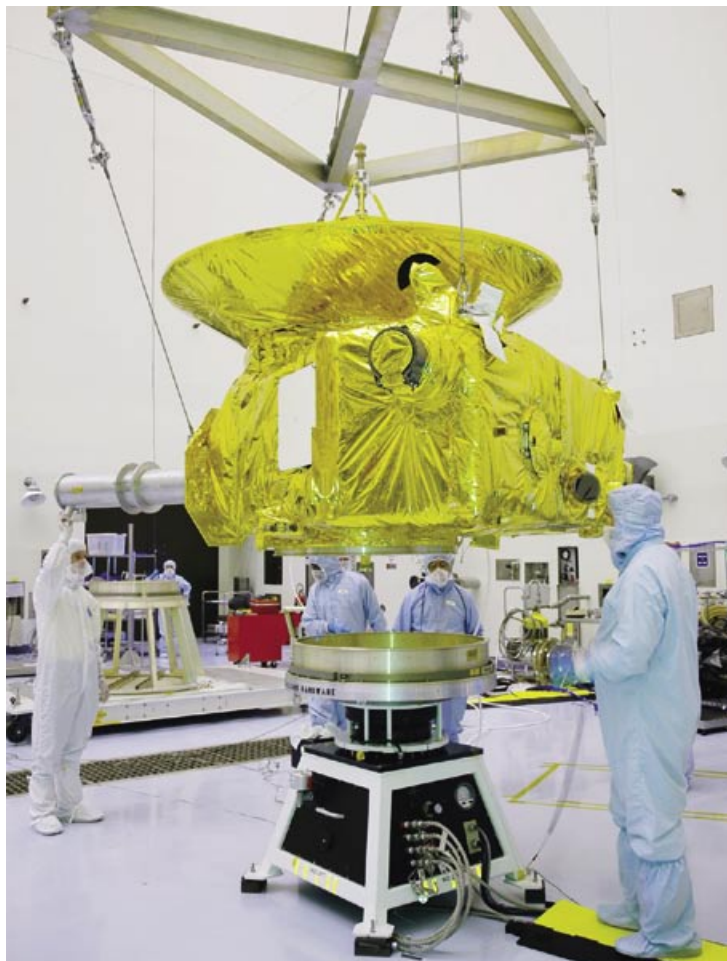
Caption: Workers, with the help of an overhead crane, lower the New Horizons spacecraft onto a spin table. The spacecraft will undergo a spin test as part of pre-launch processing.
