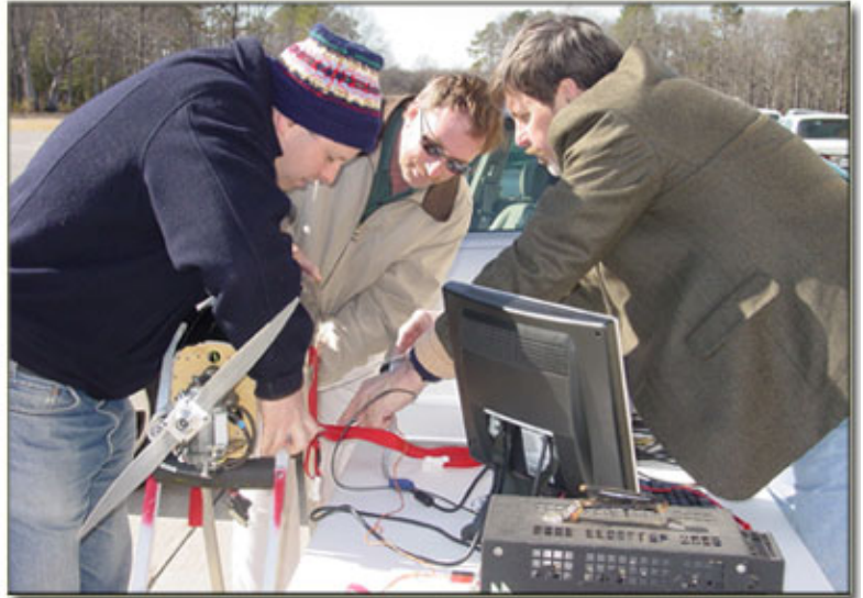
(left to right) Maurice Gonella, Aerosonde North America; Chuck Williams, NASA Wallops; and Stephen Katzberg, NASA Langley, test the GPS reflectometer in an Aerosonde UAV fuselage.
