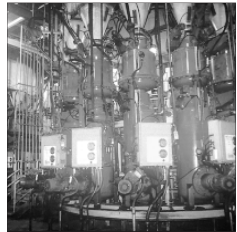
Bethlehem Steel's granular-coal injection system
