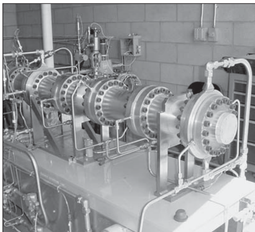
Head-end view of 10-MW gas generator
