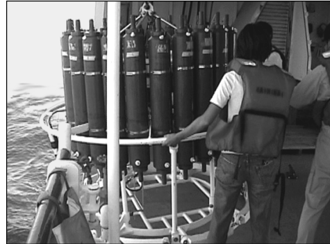
The CTS assembly is used to collect water samples and measure profiles of temperature, salinity, density, and pH versus depth.
