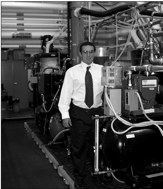
Graduate student Brian Bland, with the pilot plant he constructed in the carbon products program of West Virginia University's Department of Chemical Engineering. The plant generates up to 20 pounds of coal-derived pitch per day, the starting point for carbon foams, speciality coke, mesophase pitches, and carbon fibers.
