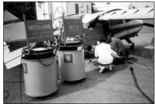
A GTC-85-72 gas turbine airplane engine was used in the LPMEOH ™ study, and demonstrated environmental benefits of the stabilized methanol.
