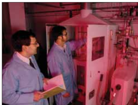
NETL's Evan Granite (foreground) and post-doctoral student Albert Presto perform experiments at NETL's bench-scale packed bed reactor, used for evaluating promising sorbents and catalysts
