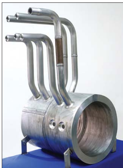
Demonstration article representing a header assembly and illustrating the fabrication processes that were successfully developed in the USC Materials Project
