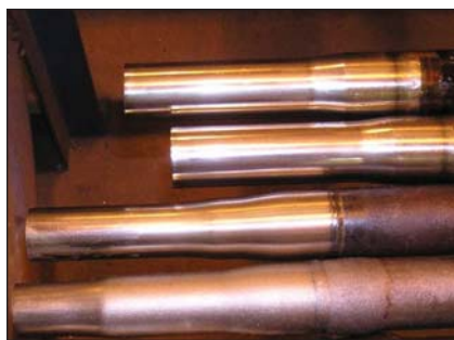
2-inch OD tube specimens (photo, left) that were sequentially swaged to 1.75-inches OD and to 1.5-inches OD (photo, right)
