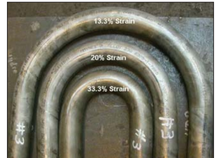
Three cold U-bends on alloy 230 produced at a North American manufacturing facility. These bends correspond to calculated outer fiber strain levels (at the extrados) of 13.3%, 20%, and 33.3%
