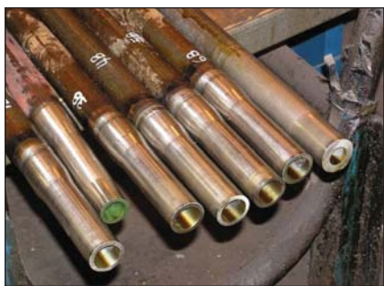
2-inch OD tube specimens (photo, left) that were sequentially swaged to 1.75-inches OD and to 1.5-inches OD (photo, right)
