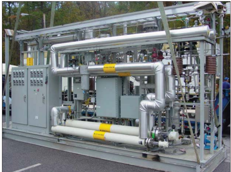
Pilot-scale DSRP system processes about 200 standard liters per minute of regeneration tailgas. The facing section shows the preheating system for the regeneration tailgas and syngas.
