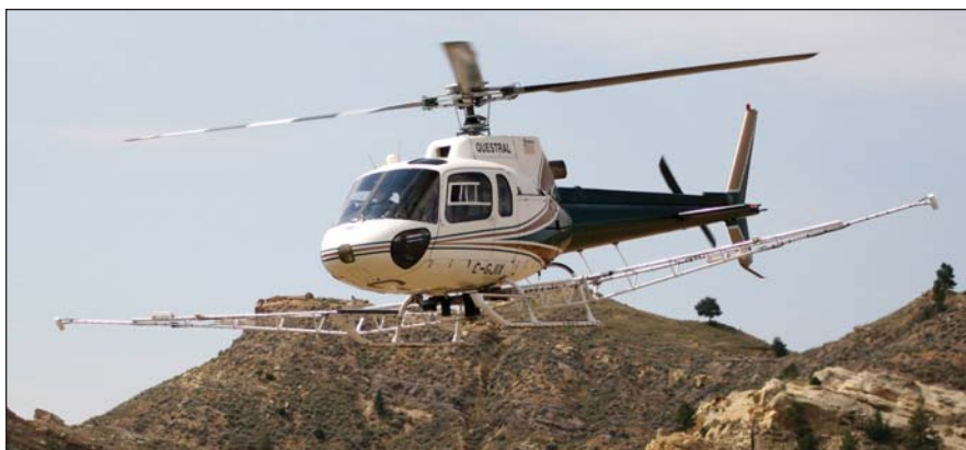
SEQUIRE's™ magnetic sensors are mounted on boom beneath the helicopter
