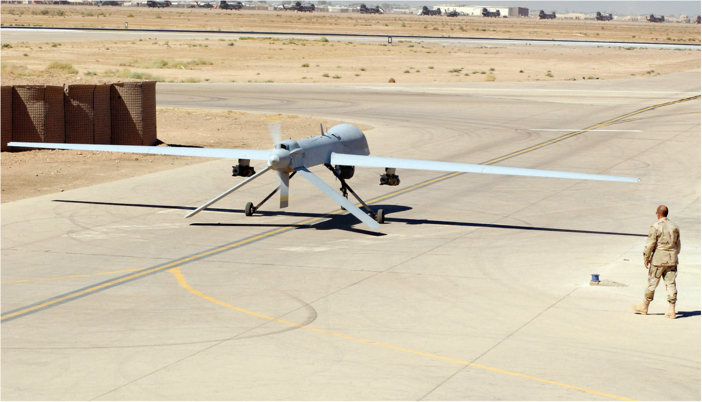
The Predator UAV, which contained nearly 15 years' worth of developmental systems funded by DARPA and private investors when it first flew in 1994, evolved out of the Gnat-750 UAV. Here, an RQ-1 Predator UAV prepares for takeoff at Balad Air Base, Iraq, on Sept. 15, 2004, in support of Operation Iraqi Freedom.
