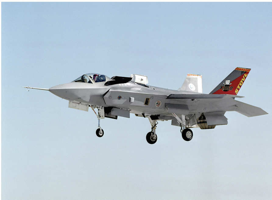
The STOVL variant of the JSF competition winner, the Lockheed Martin X-35B, boasted a shaft-driven, lift-fan arrangement that was a direct result of the DARPA research into advanced STOVL technologies.
