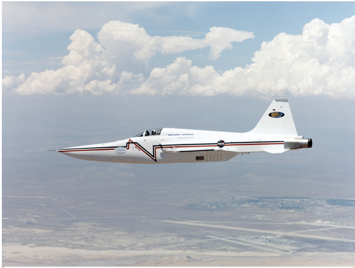
DARPA's Shaped Sonic Boom Demonstration showed that the heavily modified shape of the F-5 test aircraft also changed the shape of the aircraft's sonic boom. The research could lead to quieter supersonic aircraft.
