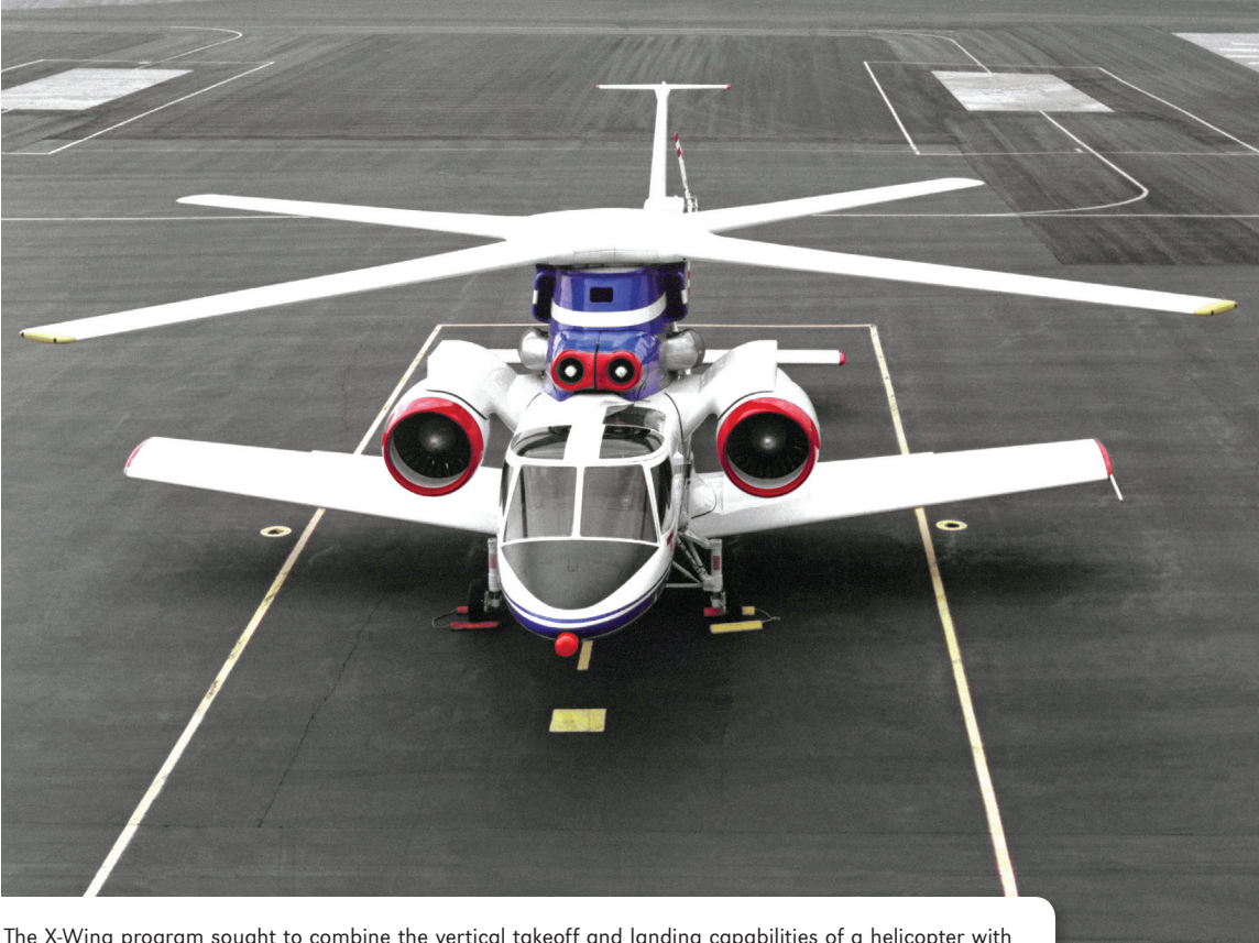
The X-Wing program sought to combine the vertical takeoff and landing capabilities of a helicopter with the high speed of a tactical jet in one aircraft.
