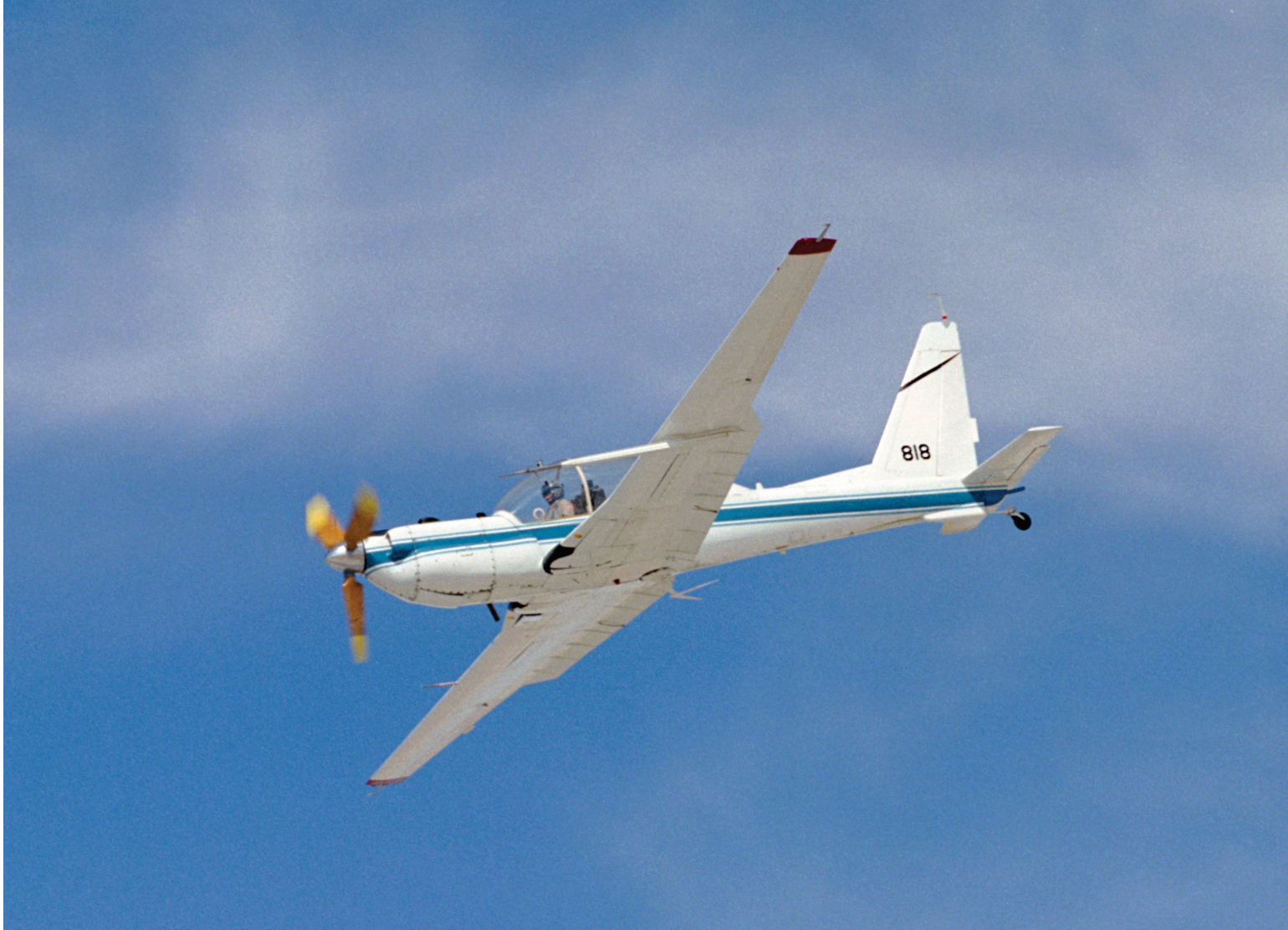
DARPA's aerospace expertise began with work on such relatively unsexy craft as the Lockheed YO-3A, pictured here being flown by NASA. The sailplane-derived wings and quiet wooden propeller are clearly shown.
