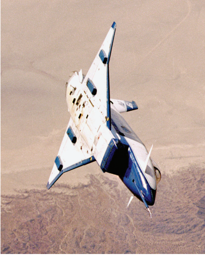
Using thrust vectoring and advanced digital flight controls, the X-31 demonstrated revolutionary maneuverability in a wide range of flight regimes.
