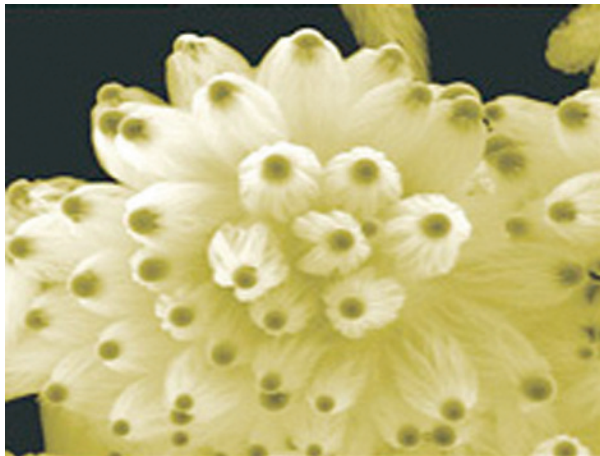
Figure 3. Example of the carrot-like morphology of \text{SiO}_x nanowire assemblies, one of five different morphologies obtained in different temperature ranges during molten-gallium-catalyzed synthesis in a three-phase reactor [6]. The gallium ball at the end of each structure is 4 to 5 microns in diameter. (Reprinted with permission from Z. Pan et al., “Temperature dependence of morphologies of aligned silicon oxide nanowire assemblies catalyzed by molten gallium,” Nano Letters 3 , 1279–1284. Copyright 2003 American Chemical Society.)
