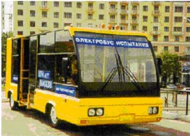
Fig. 20. Electric bus powered solely by an asymmetric electrochemical capacitor system. (Photo courtesy of ESMA Joint Stock Company)
