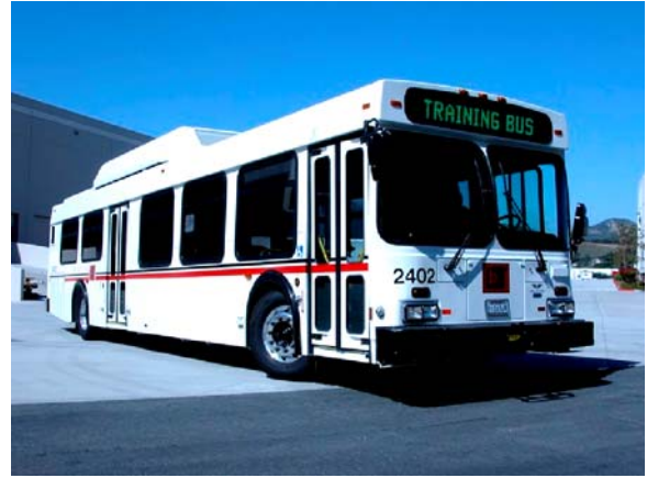
Fig. 21. Gasoline/electric hybrid bus with an electrochemical capacitor energy storage system. (Photo courtesy of ISE Corporation)
