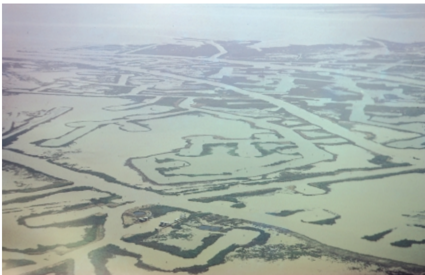
Fig. 16. An oil field in the Louisiana coastal wetlands. The extensive network of artificial canals provides access to oil and gas wells. The canals are bordered by elevated deposits of dredged materials that block the natural flow of water to the remaining wetlands.
